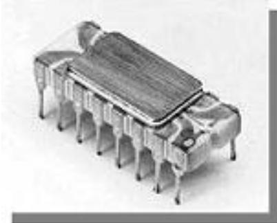
The 4004 was the first CPU created as a single integrated circuit. Created by Intel in 1972 to be used primarily in hand held calculators.
