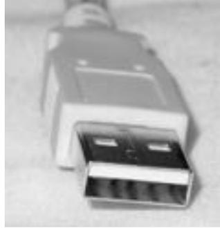
Initially USB version 1.1 supported (2) speeds 1.5 Mb/s and 12 Mb/s. The newest version, ver 2.0 supports up to 480 Mb/s. Up to 127 USB devices can be connected using hubs.
