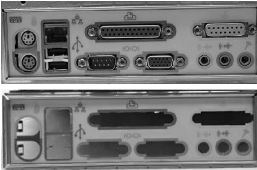
I/O shields come in various configurations to accommodate many different motherboard configurations. Shields are designed to snap into place in the rear of the system case.
