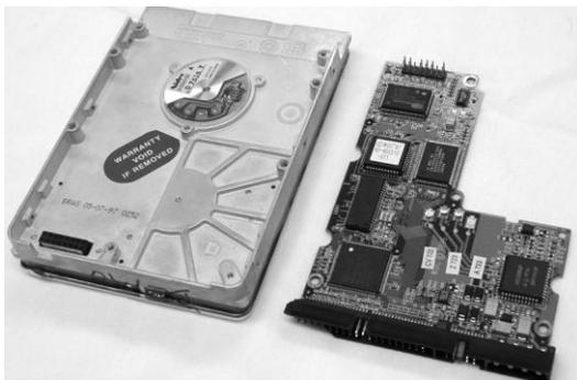
The Controller connects directly to the back of the hard drive.
