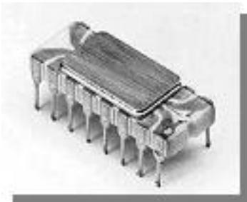
The 4004 was the first CPU created as a single integrated circuit.
