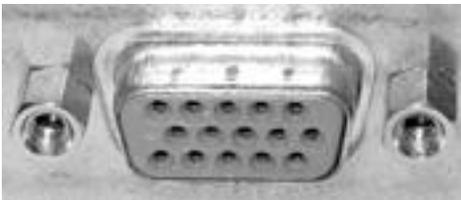
15 Pin Female, D-Shell connector is the only connector with three rows of pins.
