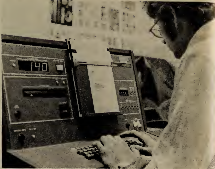
Paul Nichols types on a composing machine which is used to set type for a project he will be doing during the quarter. The machine works something like a computer in the way that it can automatically position material.
