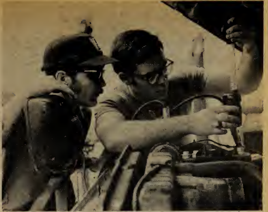
In an automotive lab, Mark Bobysud, left, and Greg Zanoni check out a battery with a hydrometer. The automotive tech program offers both one-year and two-year plans to provide students with a thorough understanding of automotive systems.
