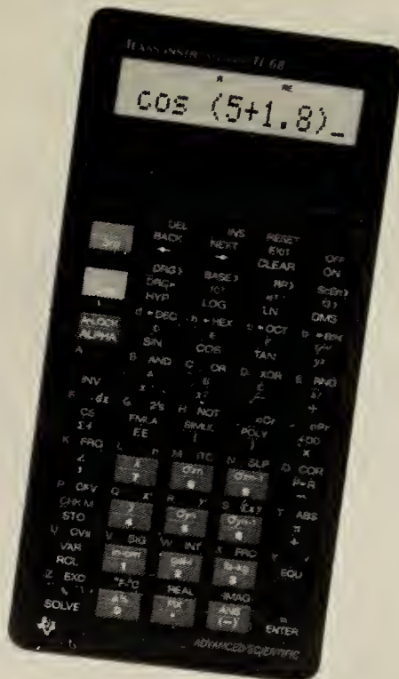
The TI-68 solves up to five simultaneous equations, performs complex number functions and offers formula programming.
