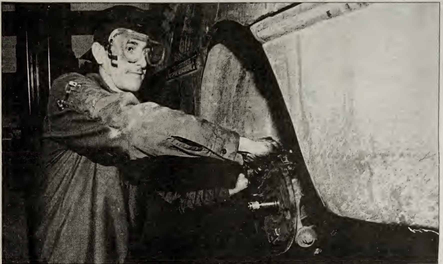
Amin Faizi does a little repair work, working on the rear drum brakes on a 1989 Ford Probe in COD's Automotive Lab, IC 0023.
