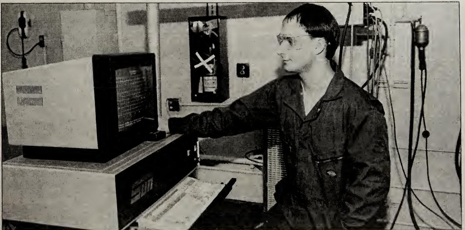
Using a Sun computer, Ken Walling checks the firing voltage of the ignition system in a Ford Escort to make sure it's correct.
