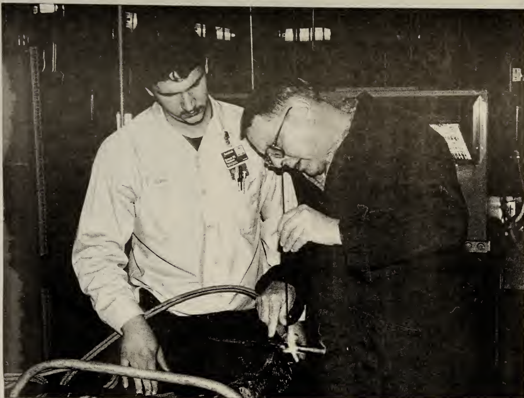
Student Ernie Toutant, aided by professor Don Carlson, constructs a braze joint using copper pipe and silver solder.
