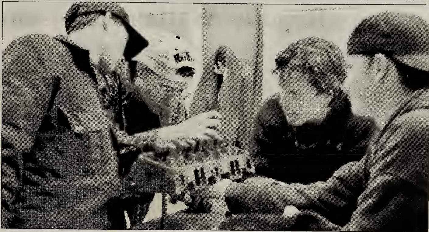
Douglas Le, Steve Delaney, Brian Kornovich and Tim Rose are resurfacing cylinder heads and valve seats during Engine Design and Repair class.
